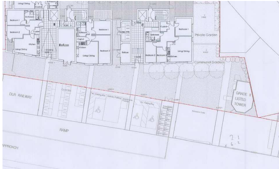
Part ground floor plan showing tapering of building in relation to the listed tower.
